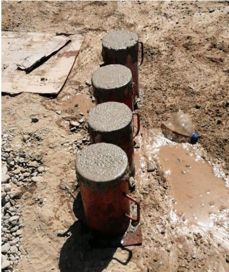
PROBETAS EXTRAIDAS DE COLUMNAS
